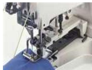
7. **Double Needle Machine.** This is used in the construction of the different kinds of clothing especially for the inseam, outseam and side seam.
